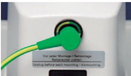
Figure. PE connection socket on the mobile stand with the green/yellow equipotential bonding conductor
