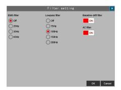
Support four kinds of filter setting: AC filter, baseline drift filter, EMG filter, lowpass filter. High-speed baseline correction filter ensures rapidly correcting the baseline
