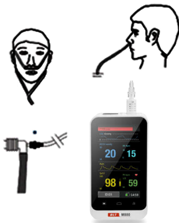
Fig 5-1-2 Connection of Sampling with CO2 3-way Stopcock or patient's nose
